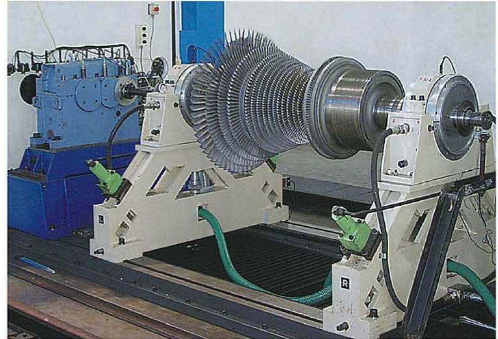
ABRO machine model HR5K (VAC) with vacuum hood open and turbine loaded on the machine.
